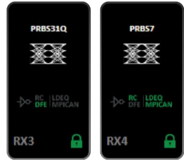
Figure 27: RX side with different EQ types enabled
