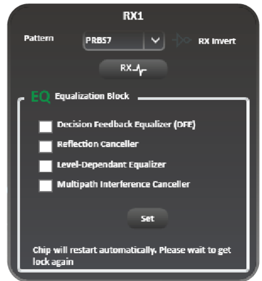
Figure 27: RX side with different EQ types enabled
