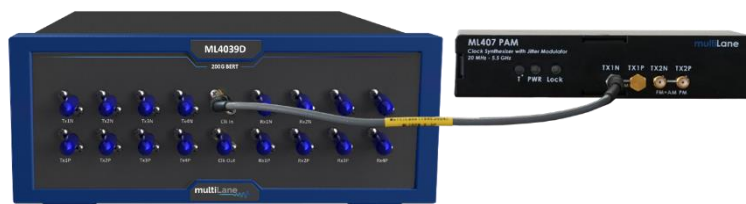
Figure 33: Jitter tolerance hardware setup
