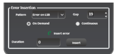
Figure 20: Error injection tab
