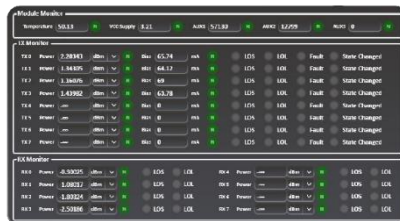
Figure 54: Digital Diagnostic Monitoring tab (DDM)
