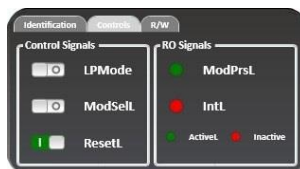
Figure 57: Controls tab of the CMIS window
